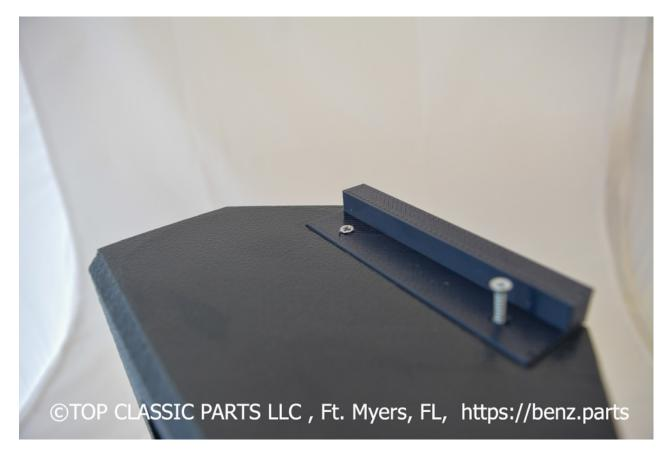
Use the Screws to fix the Support material to the Cupholder as shown in the picture
