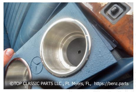
The installed Front Support for our Cupholder's goes all the way under the Shifterwood Cover of your R107 to fix the front on the installation surface.
