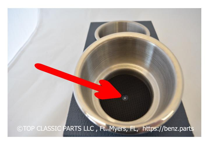
The rear cup should get fixed with the third and bigger screw in your package. Once the support is pushed as far as possible in driving direction under the Shifterwood Cover you can proceed to screw in the rear cup.
