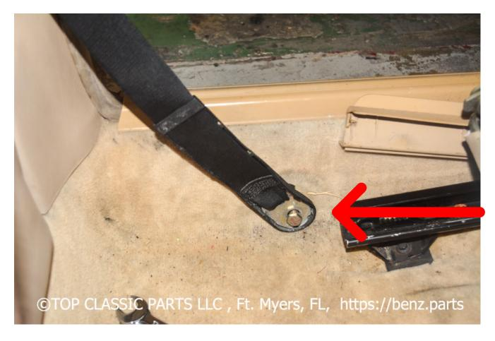
First Step is to remove the screw with a wrench – located on the sides behind the seats.
