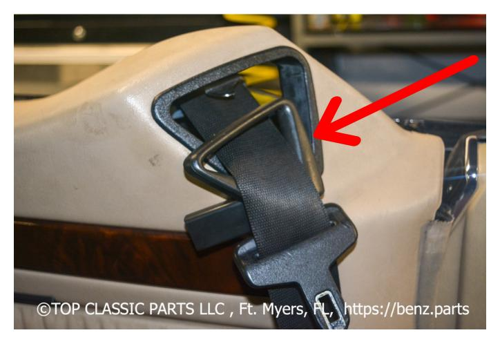
Remove the old Seat Belt Holder (inner part) by pulling it from its position.
