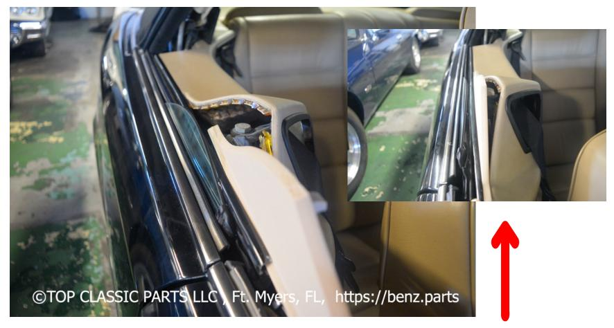
Push it all the way back so the top of the part fits to the top corner as shown above
