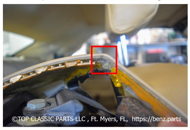
We used a small cutting plier to remove the glue
