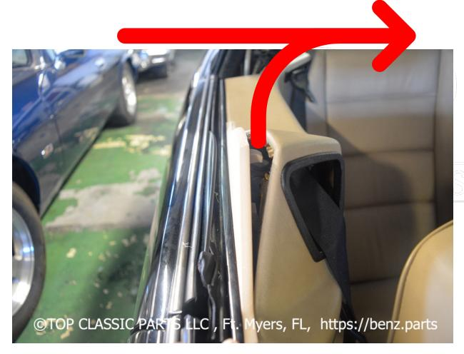
Apply glue to the clip and right on the spot where we removed the glue earlier (ref. slide 3), and along the old glued areas too.
