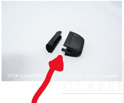
The new parts needs to be installed as shown in the picture, the clips are on the bottom and the larger part at the top
