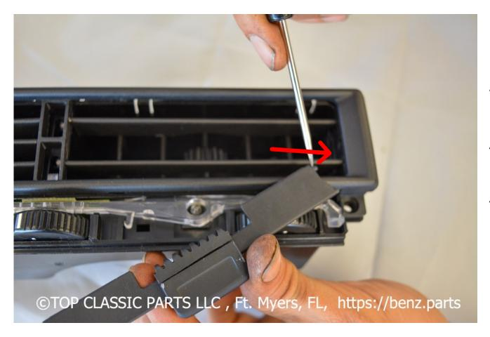
The pin must fit in the hole marked in the picture
