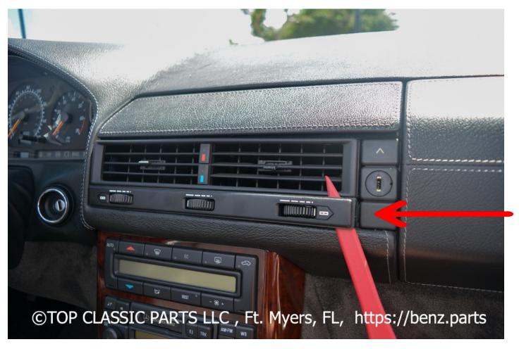
Remove the cover with a plastic wedge as shown in the picture
