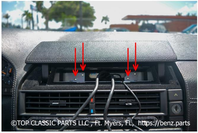
One the telephone is pulled from the compartment box, there is a metal case that was holding the phone. Remove the 4 screws as shown in the picture and pull the case from the box.
