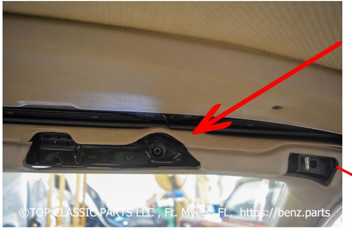
Once removed, this is the installation area for the new Soft Top Opener Covering
