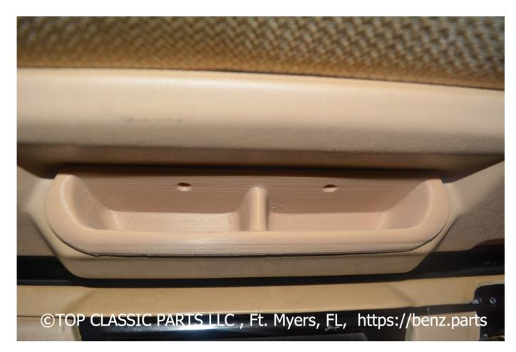
The new Grab Handle can easily be pushed in the installation area.
