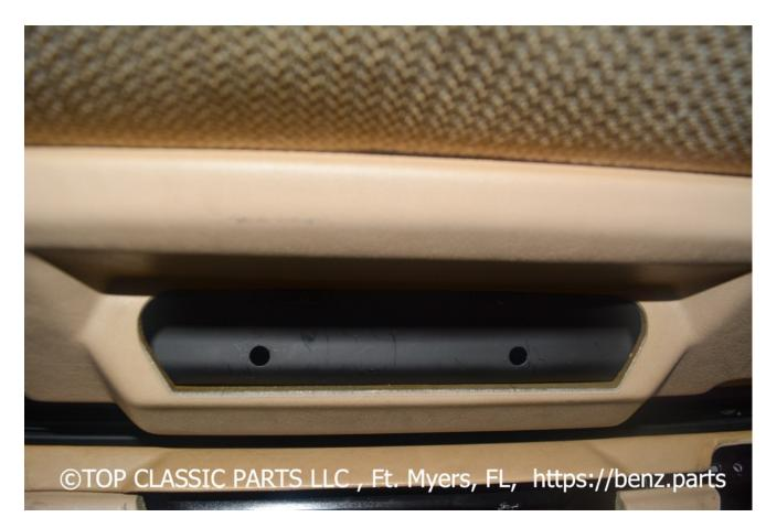
The broken grab handle can be easily removed – just take off the screws and pull the grab handle from its position.
