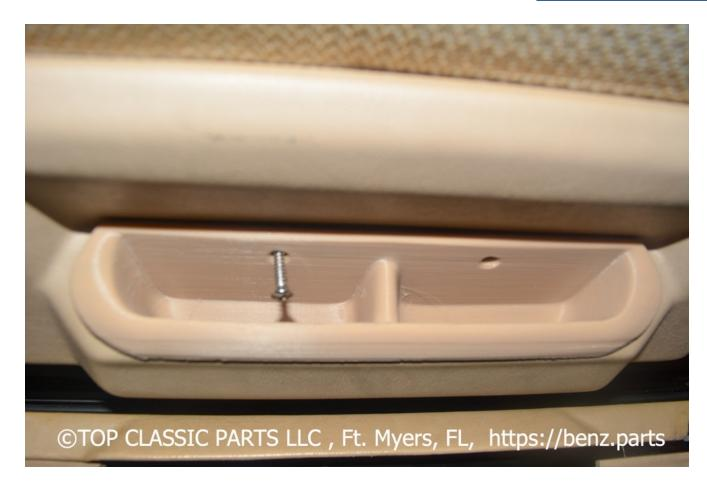
Put the screws in the holes and fix the Grab Handle in the installation area.
