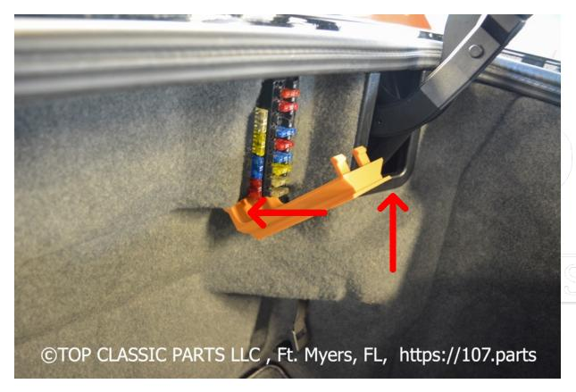
First instert the new Cover so the clips slide into the slots below the cover.
