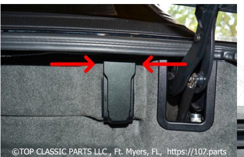
You can remove the cover by pulling it on top, shown in the picture above. See result on the following slide.
