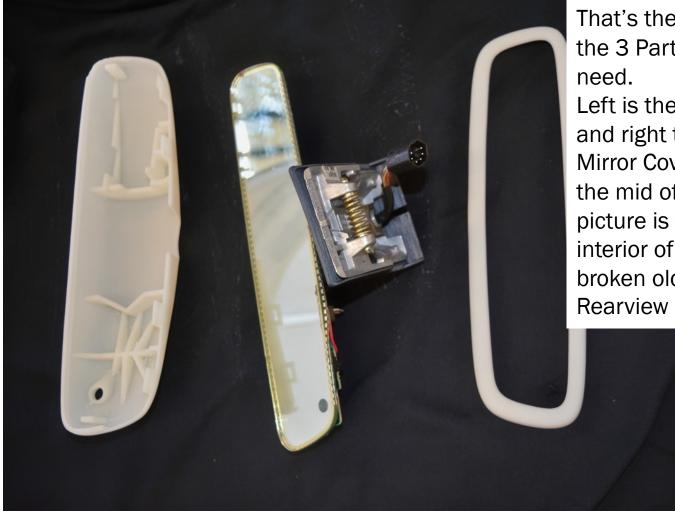
That's the view on the 3 Parts you Left is the back and right the front Mirror Cover. In the mid of the picture is the interior of your broken old **Rearview Mirror.**
