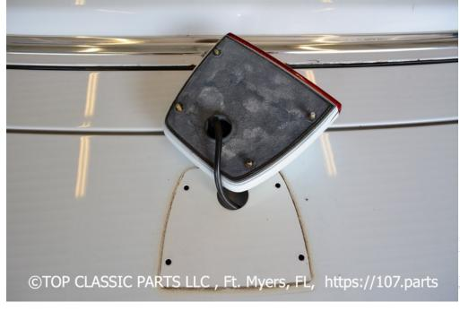
The final step is to bring put the break light back in its position and fix ii by screwing all 4 nuts back on each screw.
