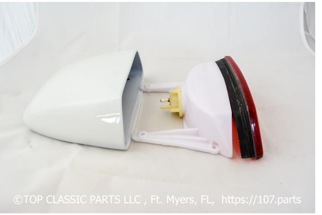
Put all the parts back together, fix the interior with the interio screws as shown on slide 4. Connect the cable to the bulb and put the rubber seal back on the bottom of the part as shown on the next slide.
