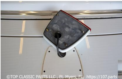
Once the exterior screws are off you can easily pull the Brake light from its position.
