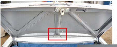
The first step is tp open the Trunk to access the screws shown in the picture below.
