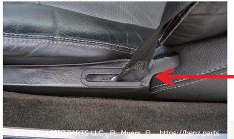
The first step is to remove the old/broken seat belt cover from the installation area. You can easily use a wedge as shown on the next slide.
