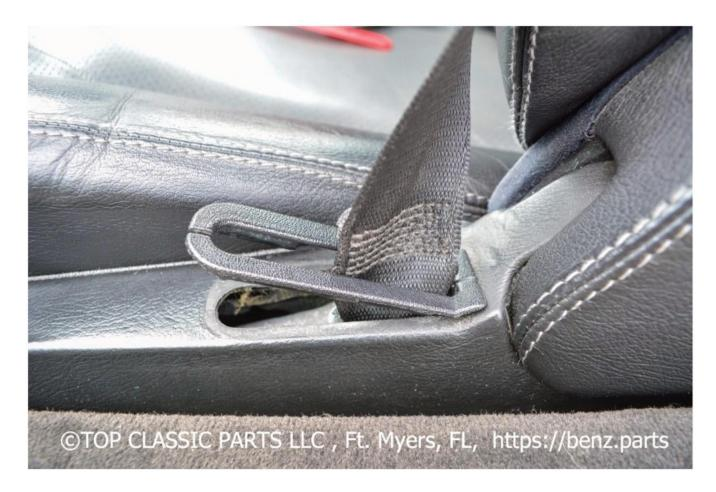
Put the new Seat Belt Cover in position as shown in the image. We recommend to fix the Cover starting with the rear side, then proceed with pushing the front side all the way down until it clicks in its position.
