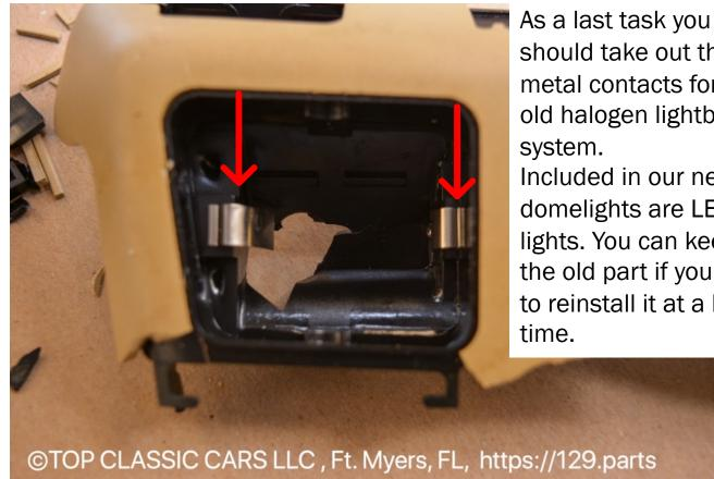
should take out the metal contacts for the old halogen lightbulb Included in our new domelights are LED lights. You can keep the old part if you want to reinstall it at a later
