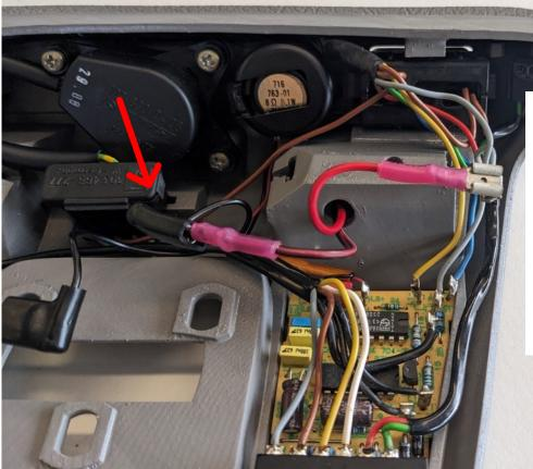
In this case the red has to be connected with the gray cable. In any of the Domelights the most important is that you connect black to black. As shown with the red arrow.
