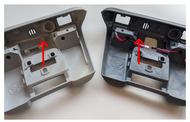
The installation for the regular 129 and the 124 Domelight are exactly the same. The only difference between the regular 129 and the SOS version is the part that you can see marked in this picture. The SOS version has the 3<sup>rd</sup> screw of the middle part on the left side instead of the right side as shown later in the HowTo.
