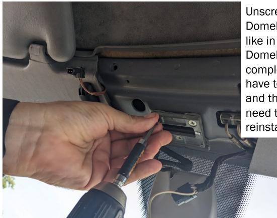
Unscrew them all, to get the Domelight off. It can happen like in this case that the old Domelight falls apart completely.. Then you'll still have to remove the 3 screws and the metal plate as we need them again later in the reinstalment
