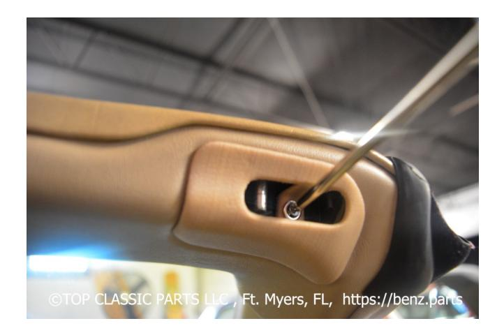
Once the Trim is in Position, use the screw in the package and a scewdriver to fix the Trim in the intended positon.
