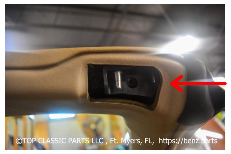
Remove the old or broken Sunvisor Trim to free the installation area as shown in the picture.
