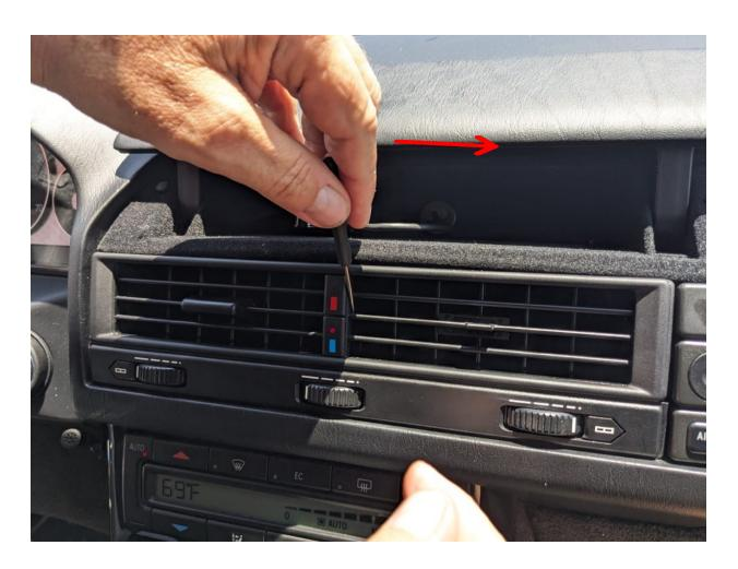
This is the quicker version of removing just the middle fin that holds the vent lever. Therefor you'll take a very small flat screwdriver and push it between the fin and the inner or middle side. Don't try it from the outer side!! Then you move the screwdriver to the right and that part should pop right out. For easier understanding check the next slide
