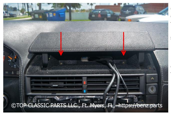
Once the metal case is removed, there are two more screws as shown in the picture. Please remove in order to pull the compartment box from its position.
