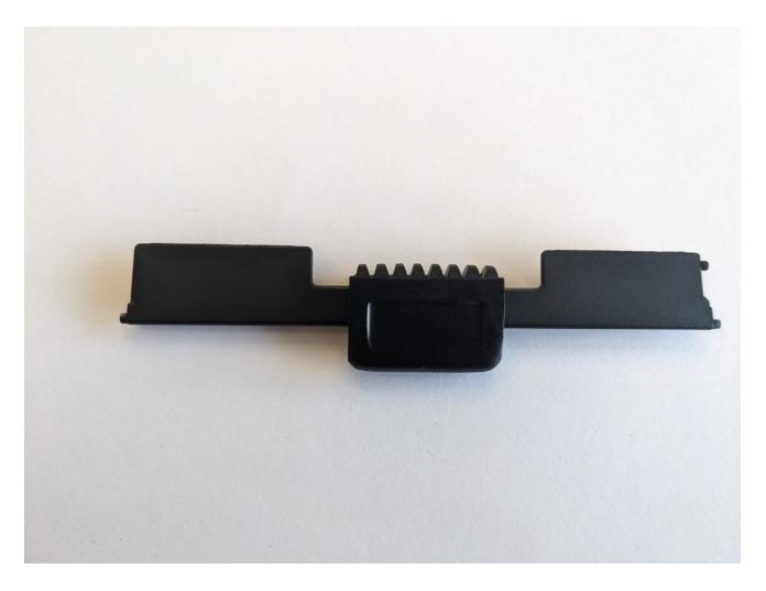
Once it clicked together make sure it moves from left to right. Before you install it back into the car, it must be positioned in the middle as pictured here.
