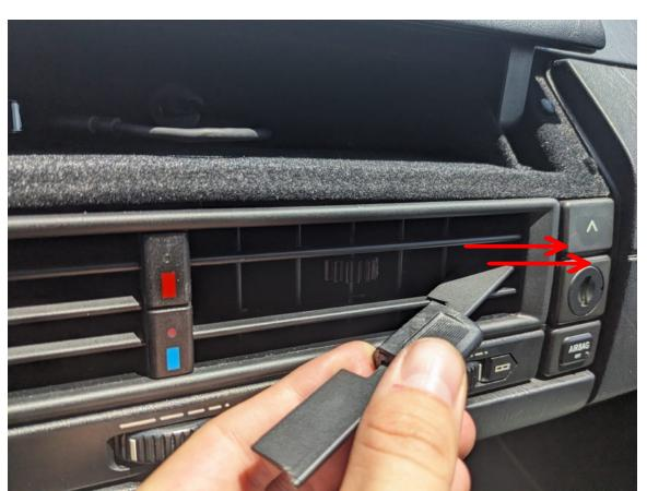
Back in the car. As a reminder, please make sure that all the fins are perfectly straight, the horizontal ones in the front as well as the vertical ones behind them. Also make sure that the lever is positioned in the middle of the fin. Then start by pushing in the right side first, make sure you hit both holes with the pins on the right side of the fin. They should be in a straight line behind each other. Then you can push in the left side of the fin
