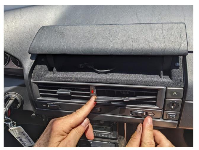
Once the inner or middle side popped out, you will be able to easily pull it out of the outer side. Make sure all the fins are vertically and horizontally very straight.
