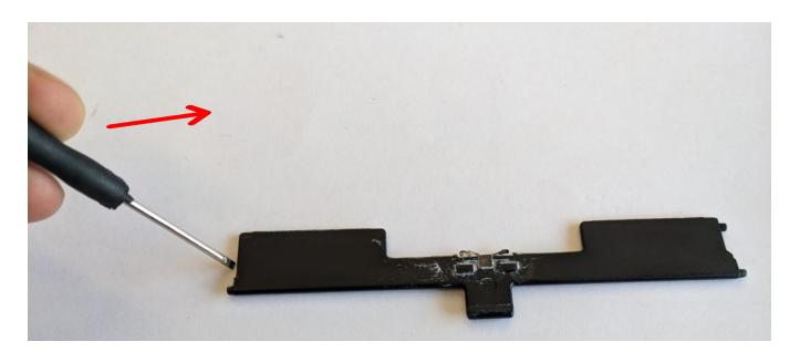
In the picture above you can see where you should place your screwdriver. Between the fin and the plastic. And then move the screwdriver in the direction of the arrow. As soon as the pin in the front of the fin pops out you can remove the whole fin. Pictured in the next slide
