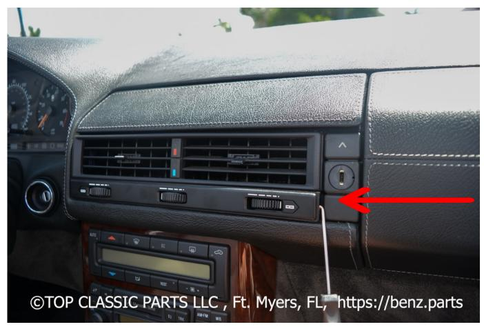
This is the installation area – The center Vents need to be removed.
